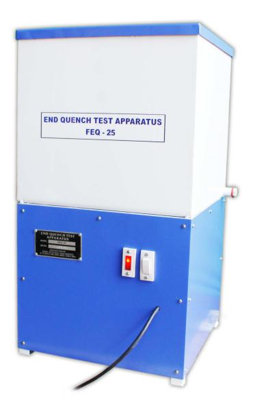
This apparatus is useful for determining the hardenability of steels by End Quench Test. The test consists of heating a standard size specimen to a given temperature for a specific period of time, followed by a water quenching at one end under specified conditions and measuring the hardness at various points from quenched end along the length of piece.
